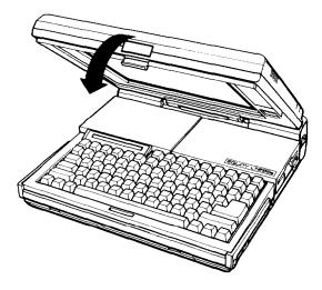
To open the screen, press the latch release button in the center of the computer (shown below). Then lift the screen back. You can position the screen at a variety of viewing angles.
